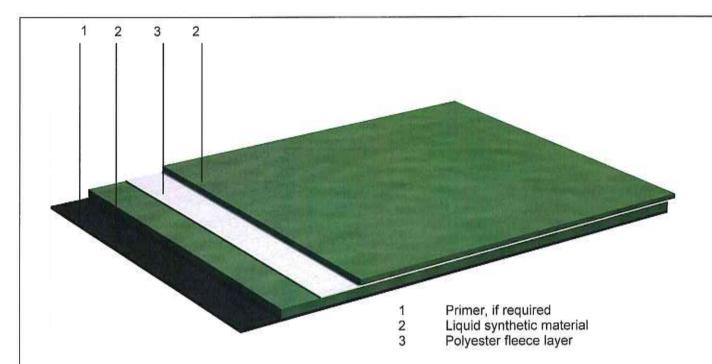
Applicable to the roof waterproofing "Triflex ProTect":
