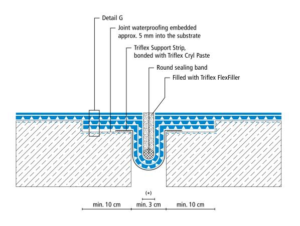
(\*) Omission of surface coating and wearing layer (see system description) (\*\*) Triflex Special Fleece or Triflex Special Fleece PF Height differences where the fleece overlaps are exaggerated.
