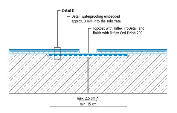
(\*) Omission of surface coating and wearing layer (see system description) (\*\*) Triflex Special Fleece or Triflex Special Fleece PF Height differences where the fleece overlaps are exaggerated.
