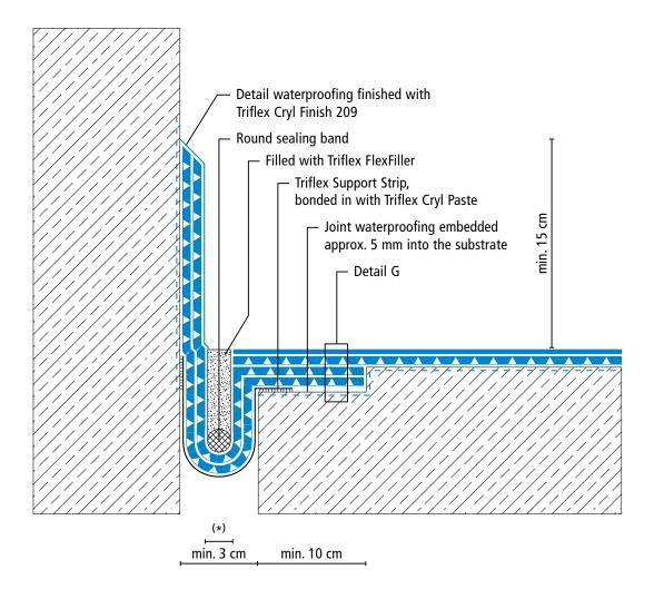
(\*) Omission of surface coating and wearing layer (see system description) (\*\*) Triflex Special Fleece or Triflex Special Fleece PF Height differences where the fleece overlaps are exaggerated.
