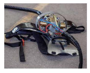
Outside the mobile unit, the mixing element and spray gun, including the selected nozzle, are used. The mixing unit is connected to the mobile unit by a hose, which contains five feed lines for conveying the following components from the machine to the mixing unit:
